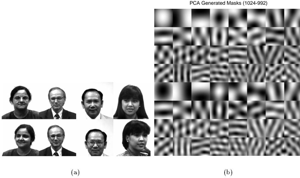
Figure 1: (a) Some sample input training images and their corresponding test images. (b) The set of globally learned PCA masks generated from training of  $32 \times 32$  window of  $128 \times 128$  size face images.
