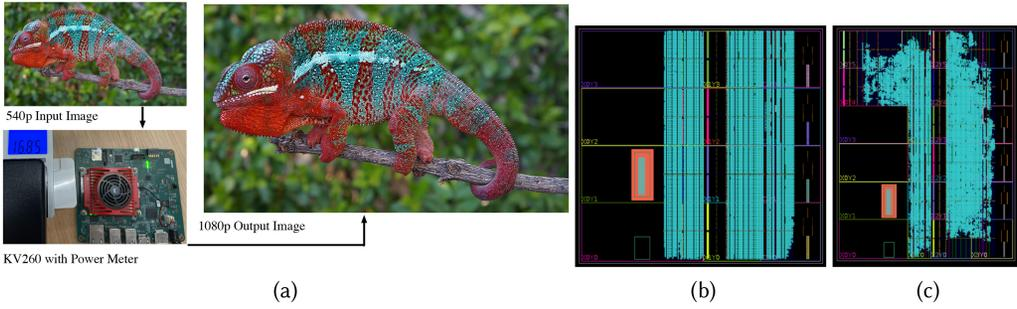
Fig. 13. (a) 540p  $\rightarrow$  1080p SR running on KV260 with a power meter monitoring the power consumption; (b) Physical implementation on KV260; (c) Physical implementation on ZCU104.
