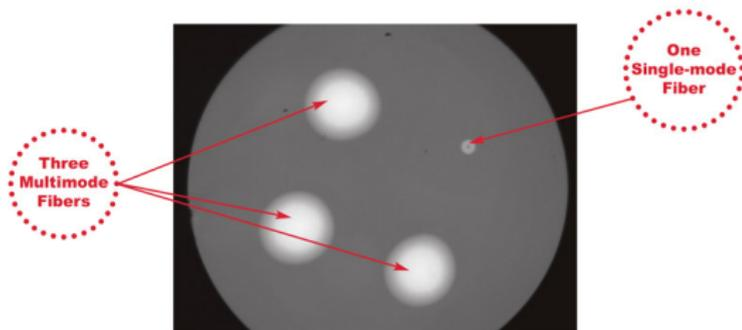
Figure: SDM using Multicore or Multimode Fiber<sup>2</sup>
