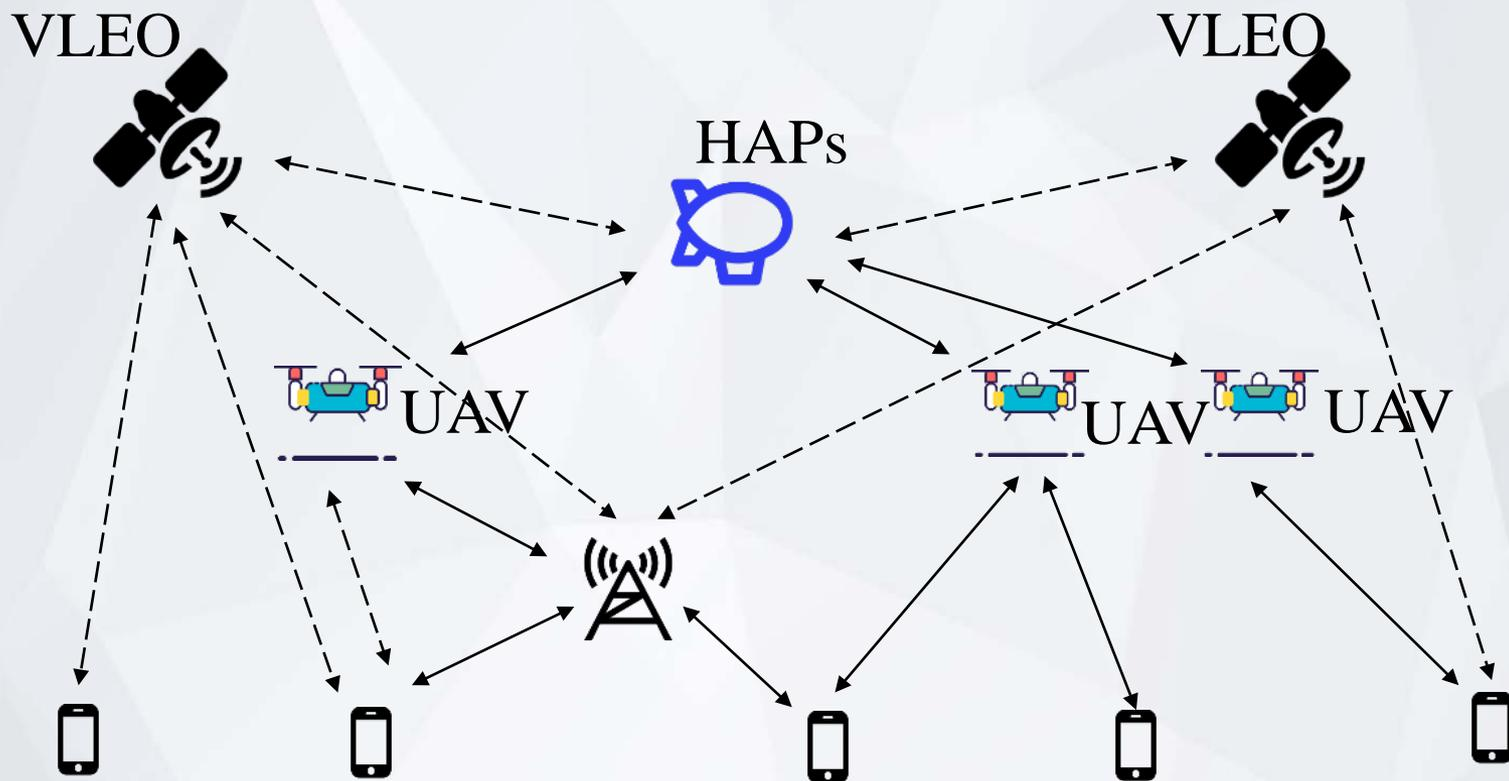
Integrated 6G network with UAV、HAPs and VLEO satellites
