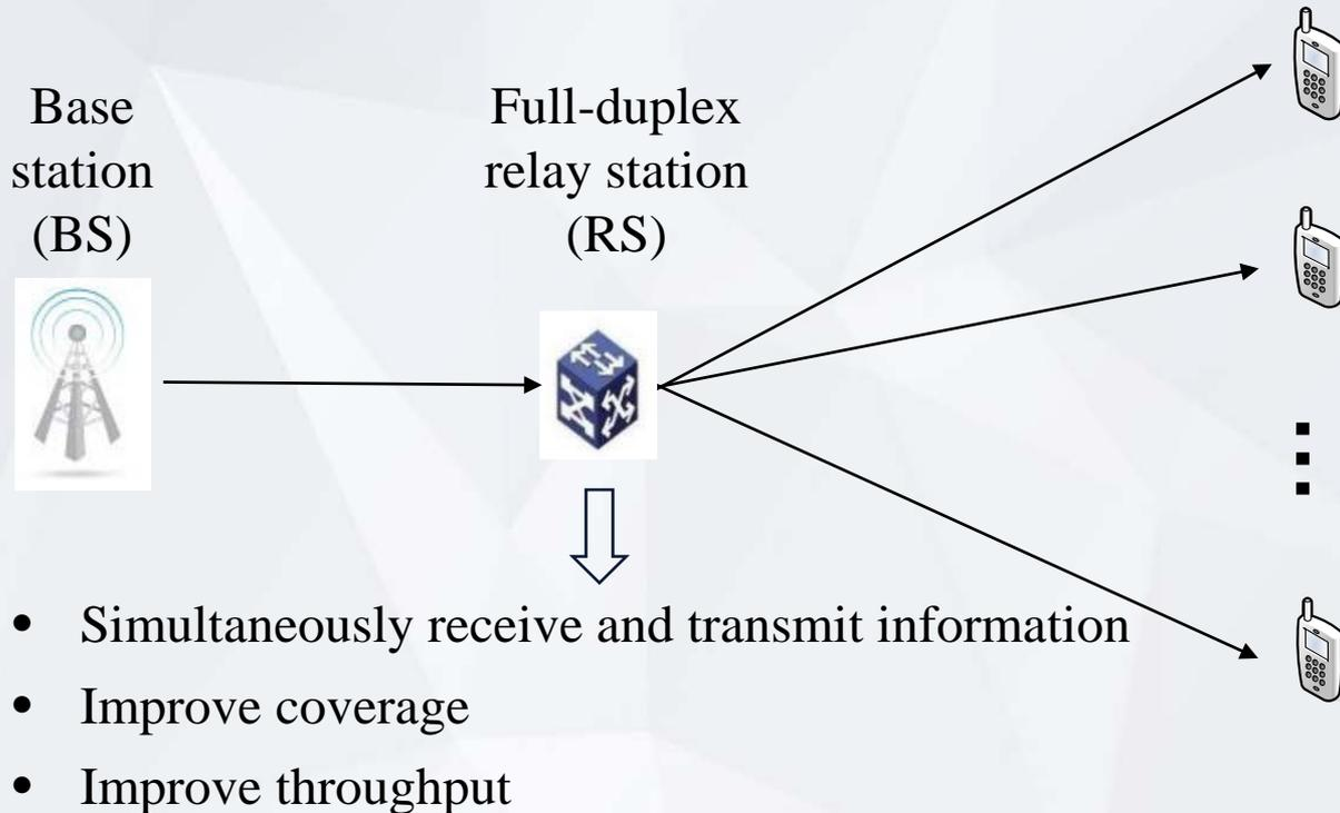
**IEEE 802.16j** and **3GPP LTE-Advanced** have proposed *two-hop relay networks* for the sake of simplicity and explicitness of system design.
