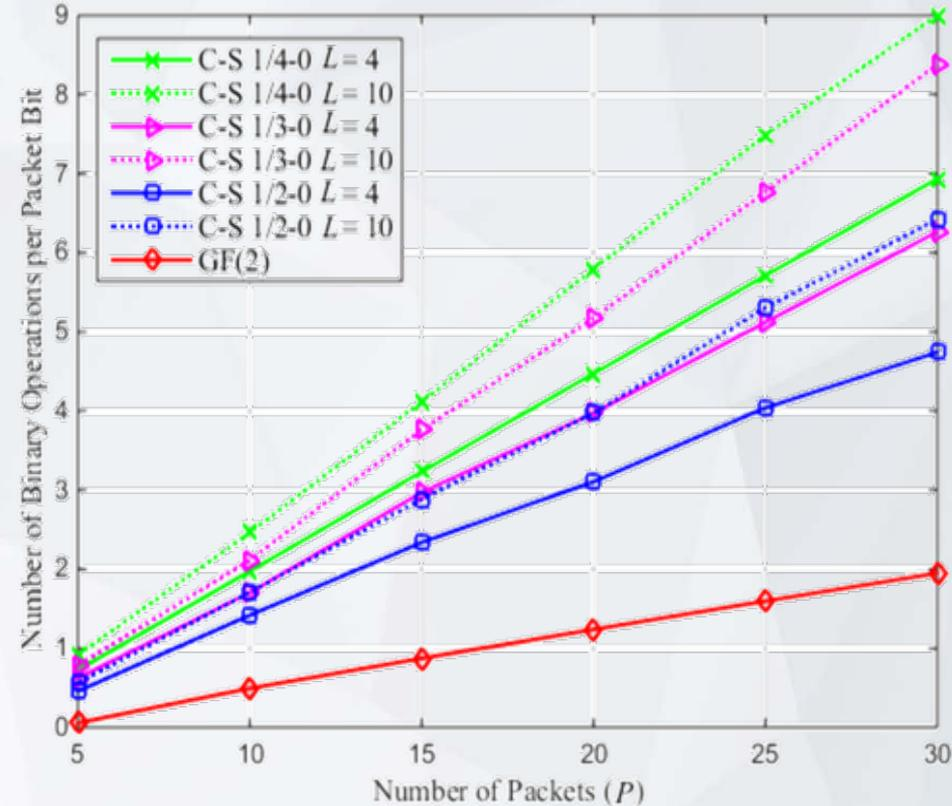
**A better trade-off:** For the case  $L = 4$ ,  $p_z = 1/4$ , when  $P \geq 15$ , # decoding operations of C-S RLNC is about **3 times** # decoding operations of **GF(2)-RLNC**, while its completion delay is within **5%** higher than **perfect RLNC**.
