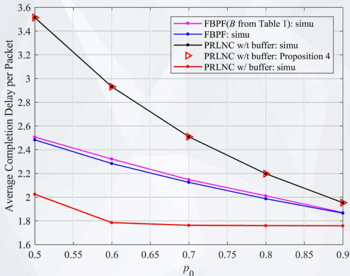
The difference between the system completion delay of FBPF for the case that  $B$  is prescribed by Table 1 and that for the case  $B = \infty$  is within **2%**.
