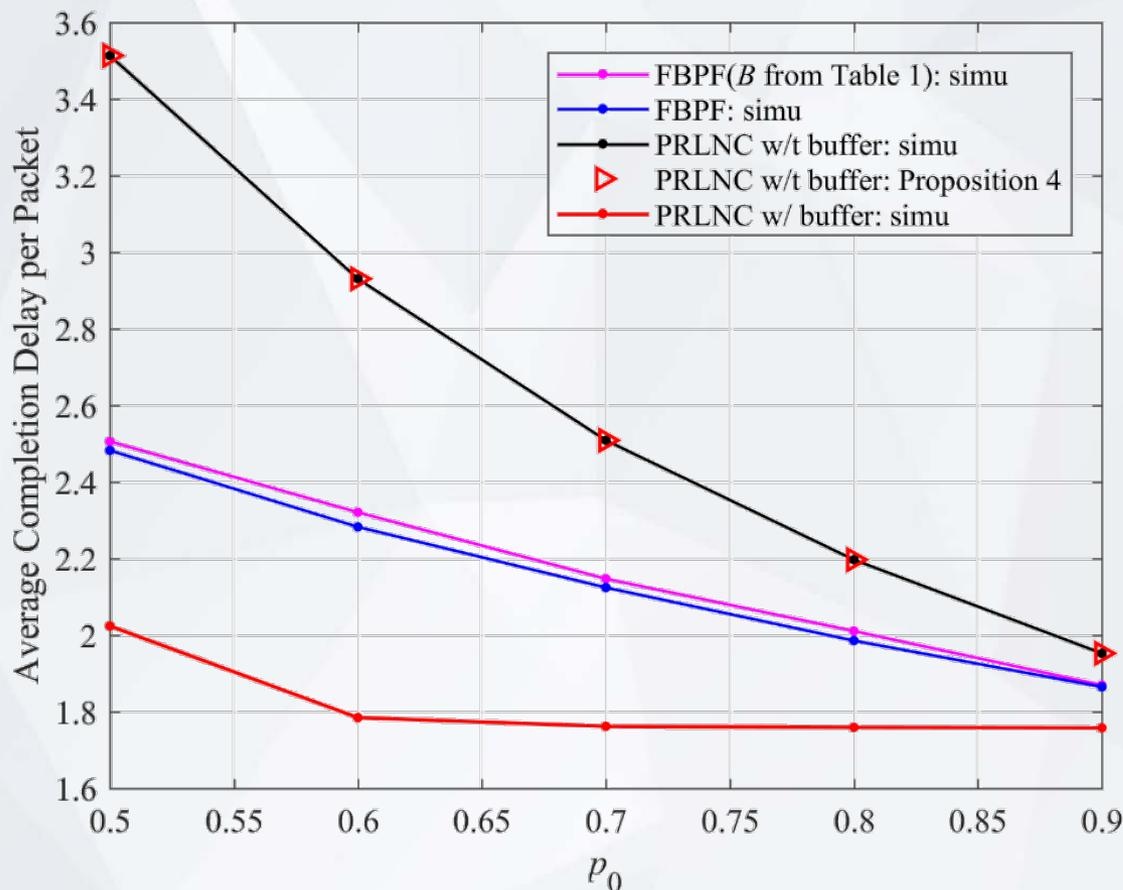
The average completion delay of FBPF is upper bounded by that of **perfect RLNC without buffer** and lower bounded by that of **perfect RLNC with buffer**.
