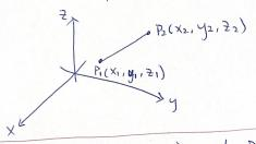
Distance between  $P_1(x_1, y_1, z_1)$  and  $P_2(x_2, y_2, z_2)$  is  $|P_1P_2| = \sqrt{(x_2 - x_1)^2 + (y_2 - y_1)^2 + (z_2 - z_1)^2}$
