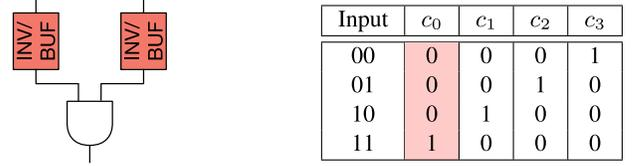
Fig. 3. Example of the camouflaged netlist and the truth table for all the possible functionalities.
