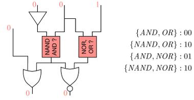
Fig. 2. Example of the camouflaged netlist.
