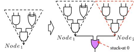
Fig. 11. Insert AND-type tree structure to the circuit (Node<sub>2</sub> is stuck-at-0 to guarantee the functional correctness).
