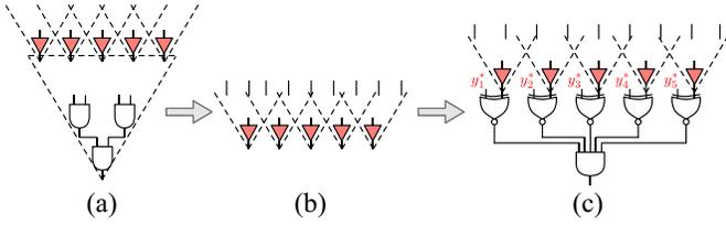
Fig. 8. Exact calculation of  $\Pr_{i \sim I}[f_{y^*}(i) = 1]$ : (a) original tree structure; (b) fanin cone extracted for all the tree input pins; and (c) form the circuit that connects all tree input pins to the desired logic values, i.e.,  $\{y_1^*, y_2^*, y_3^*, y_4^*, y_5^*\}$ . By forcing the output of the formed circuit to 1, we can solve the logic values for the circuit primary inputs iteratively as in Algorithm 1.
