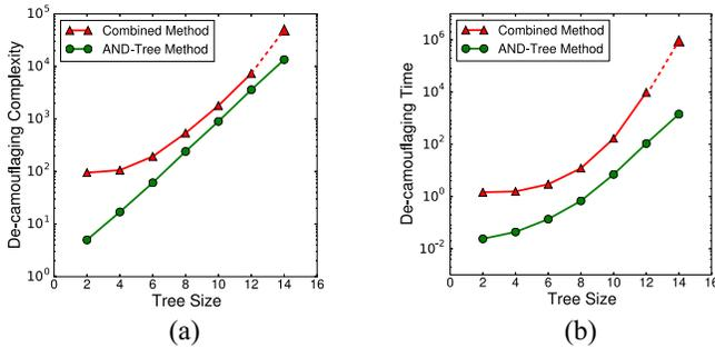
Fig. 17. Verification of the effectiveness of combining the proposed two camouflaging techniques on benchmark c880: comparison on (a) de-camouflaging complexity and (b) de-camouflaging time (dotted line indicate extrapolation).
