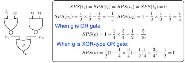
Fig. 12. SPS-based functional attack: when  $g$  is OR gate,  $SPS(o) = \frac{5}{16}$  and when  $g$  is XOR-type camouflaging cell, whether  $g$  works as an OR gate or a NOR gate are equally possible for the attacker [27], and thus  $SPS(o) = 0$ .
