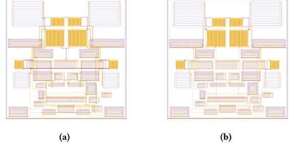
**Figure 6: GeniusRoute and AnalogFold routing solutions.**
