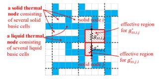
**Figure 4:** 2RM model with discretization of  $4 \times 4$  basic cells.
