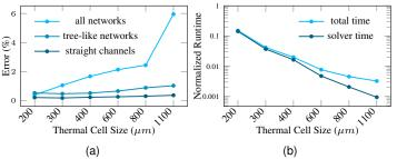
Figure 9: (a) Accuracy of 2RM compared to 4RM. (b) Speed-up of 2RM relative to 4RM.
