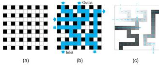
**Figure 2:** (a) Discretized channel layer where a basic cell either is TSV (black) or may be used for microchannels (white). (b) A cooling network. (c) Pressure and flow rate distribution where longer arrows represent larger flow rates and darker liquid cells have higher pressures.
