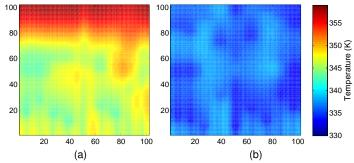
**Figure 10:** Temperature results on bottom source layer of case 1 for (a) pumping power minimization (Problem 1), and thermal gradient minimization (Problem 2).
