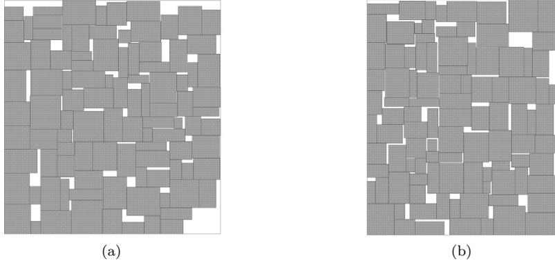
Figure 4.4: Floorplan visualizations of the n100 netlist of GSRC benchmark: (a) n100 floorplan by simulated annealing; (b) n100 floorplan by our agent. The dead space of the floorplan by our agent is lower (7.95%) compared to that (8.88%) by Simulated Annealing.
