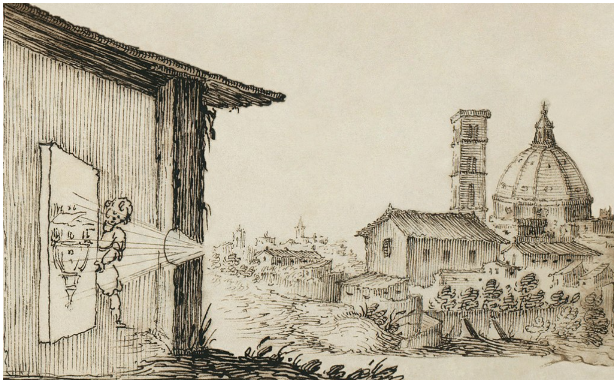
Illustration of a camera obscura from Sketchbook on military art, including geometry, fortifications, artillery, mechanics, and pyrotechnics (17th century)
