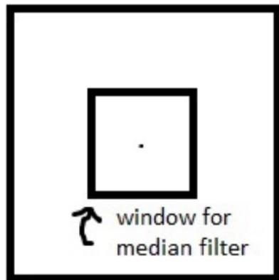
Take a window with center at pixel  $(x_0, y_0)$ . Update the pixel value at  $(x_0, y_0)$  from  $I(x_0, y_0)$  to  $\tilde{I}(x_0, y_0) = \text{median}(I \text{ within the window})$
