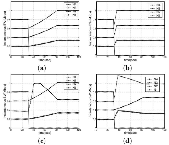
Fig. 9. Instantaneous bandwidth allocations: (a)  $\vec{\delta} = [0.01, 0.01, 0.01, 0.01]$ ; (b)  $\vec{\delta} = [0.1, 0.1, 0.1, 0.1]$ ; (c)  $\vec{\delta} = [0.01, 0.01, 0.1, 0.01]$ ; (d)  $\vec{\delta} = [0.01, 0.1, 0.01, 0.1]$ .
