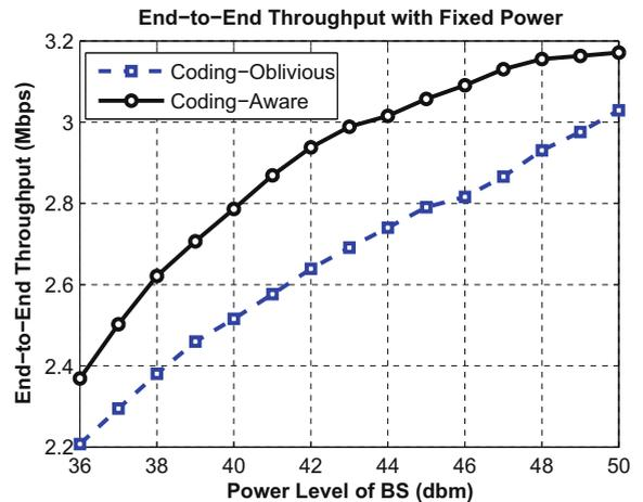
Fig. 23. BS power VS end-to-end throughput: fixed power allocation.
