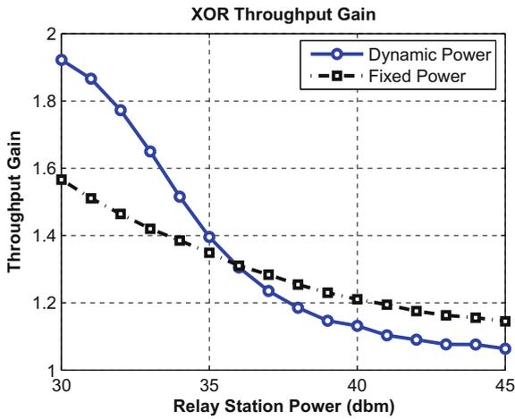
Fig. 15. RS power VS throughput gain.
