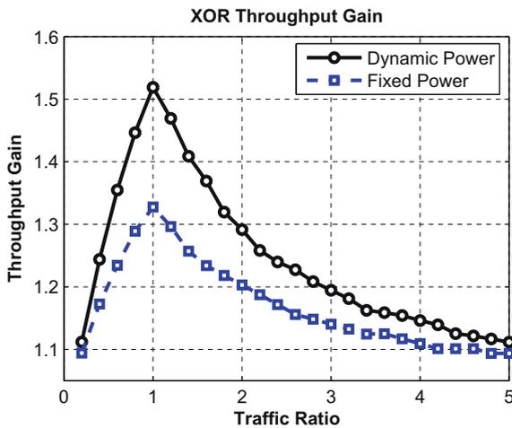
Fig. 11. Traffic ratio VS throughput gain.
