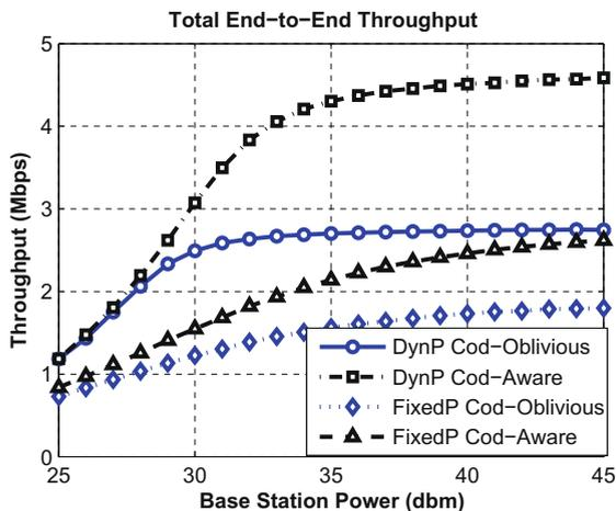
Fig. 12. BS power VS aggregate end-to-end throughput.
