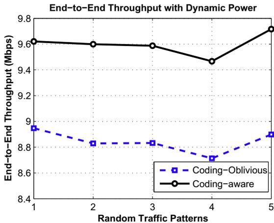
Fig. 28. End-to-end throughput with dyn. power allocation.
