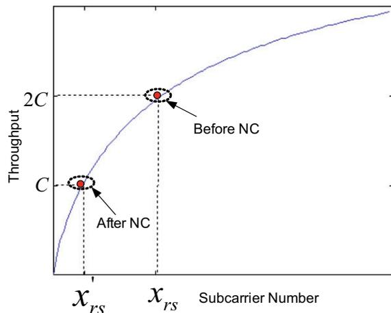
Fig. 9. An illustration of the coding and power gain.
