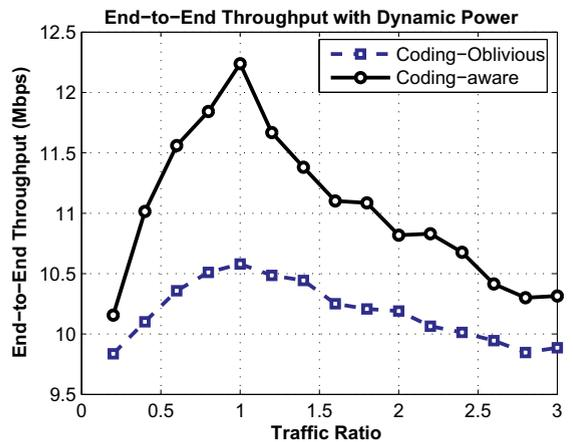
Fig. 26. Traffic ratio VS end-to-end throughput: dynamic power allocation.
