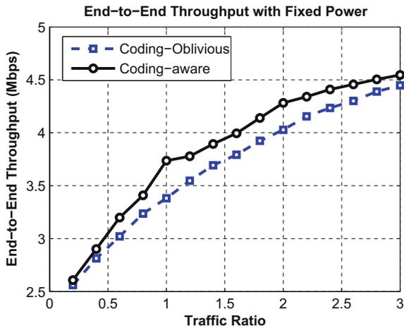
Fig. 25. Traffic ratio VS end-to-end throughput: fixed power allocation.
