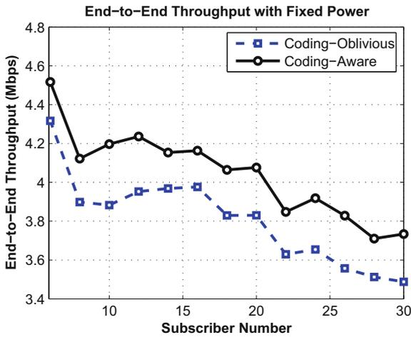
Fig. 21. Subscriber number VS end-to-end throughput: fixed power allocation.
