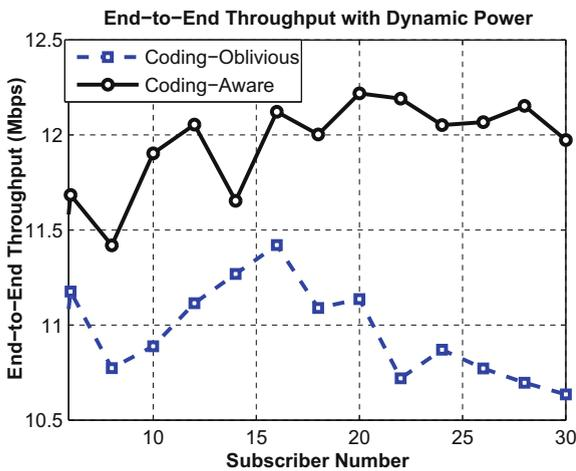
Fig. 22. Subscriber number VS end-to-end throughput: dynamic power allocation.
