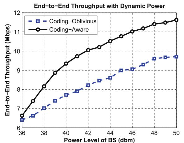
Fig. 24. BS power VS end-to-end throughput: dynamic power allocation.
