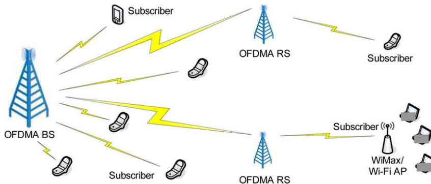
Fig. 3. Topology of an OFDMA relay network.
