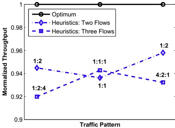
Fig. 17. Heuristics versus optimum: fixed power scheduling.
