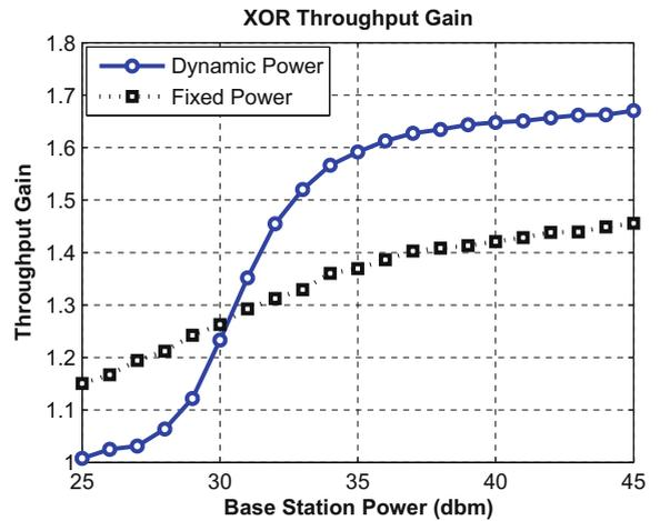
Fig. 13. BS power VS throughput gain.
