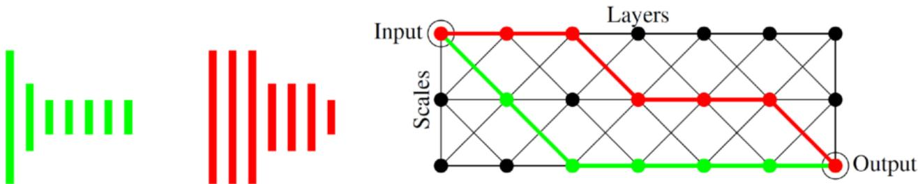
Figure: Fabrics embedding two 7-layer CNNs (red, green).
