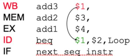
Need to forward from the EX/MEM pipeline stage to the ID comparison hardware for cases like
