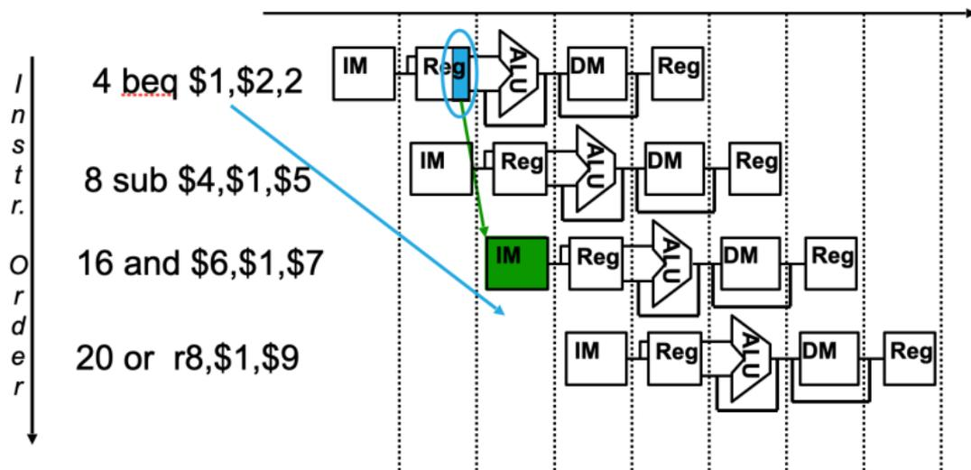
To flush the IF stage instruction, assert `IF.Flush` to zero the instruction field of the IF/ID pipeline register (transforming it into a nop)
