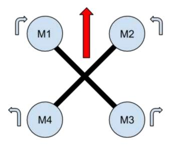
In our design, X layout of quadcopter is used. Assuming the head of the quadcopter is north. Motors M1 and M2 are the front motors, and motors M3 and M4 are the rear motors. M1 and M3 are spinning clockwisely, M2 and M4 are spinning anti-clockwisely.
