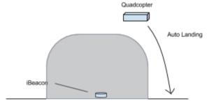
get the approximate distance from the iBeacon. So if the quadcopter is out of certain distance or the iBeacon is turned off, the quadcopter will trigger the auto
