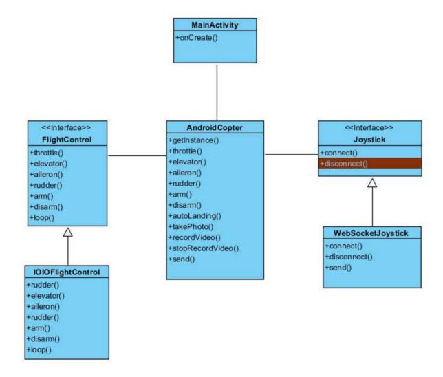
MainActivity is an Android Activity object. An AndroidCopter object can be created by calling getInstance() method. An AndroidCopter object has a FlightControl object and a Joystick object and both of them are interfaces. Currently, we have implemented IOIOFlightControl and WebSocketJoysitck, so that the android application can send control signal to quadcopter and we can control it via WebSocket.
