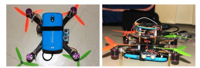
230mm quadcopter frame is used for the project. The mobile phone is installed below the frame, this installation can capture clearer photo. The IOIO board is installed on the frame.
