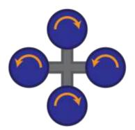
To adjust the altitude of the copter which makes the copter go up or down, it is controlled by turning up or turning down the speed of all rotors.
