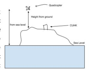
measured by barometer is the distance from the sea level.
