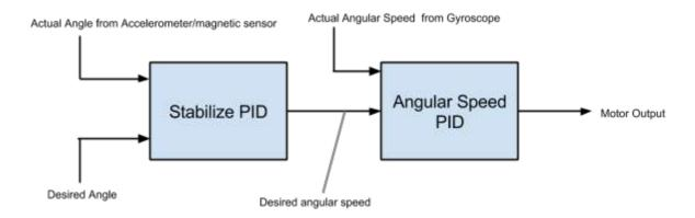
The actual angle of X-axis and Y-axis can be obtained from the accelerometer and Z-axis is obtained from the magnetic sensor. Furthermore, the quadcopter can go forward/backward/left/right by changing the desired angle input, Combining everything, the code in the Android Applications like this:
