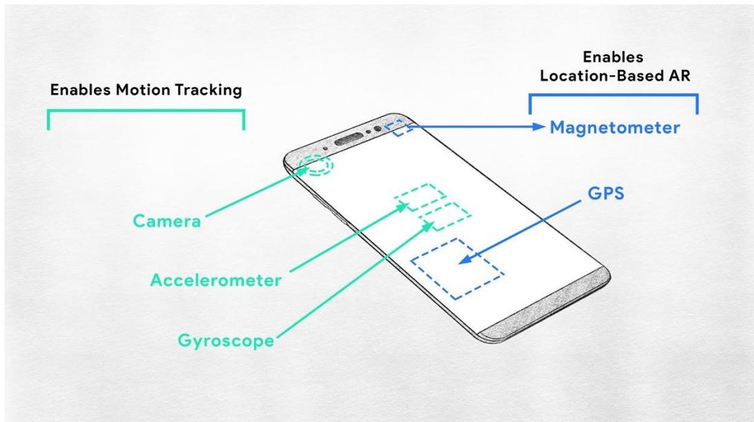
Figure 5-3 Hardware of mobile phone enhancing the motion tracking
