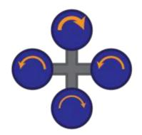
To adjust the roll of the copter which makes the copter go to left or right, it is controlled by turning up the speed of one rotating rotor and turning down the speed of rotor on the opposite side.
