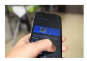
After the stabilization algorithm was finished, to ensure the correctness of output values of motors, these values were printed on screen first instead of putting the phone on the quadcopter. Then we could shake or move the phone to see whether the output values are correct or not.
