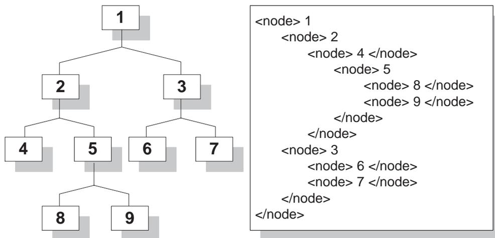
**Figure 2.4:** A tree structure and its corresponding XML data describing its structure
