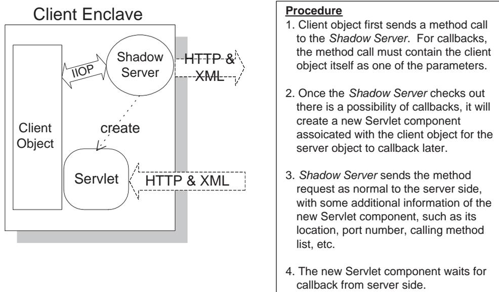
**Figure 3.5:** CORBA callback mechanism on client side
