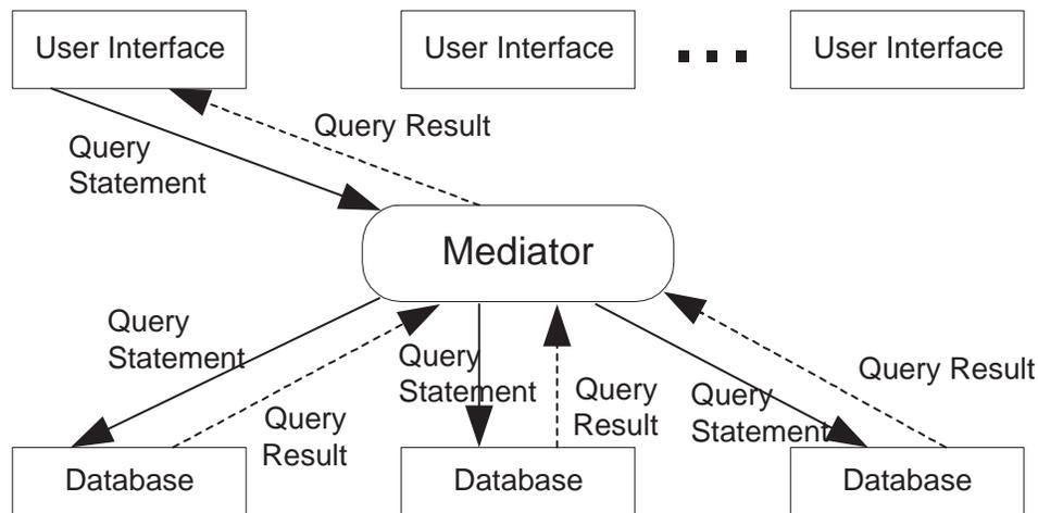
**Figure 6.1:** Diagram of the mediator concept
