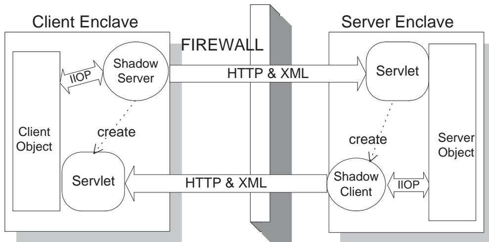
**Figure 3.4:** Mechanism that supports CORBA callbacks
