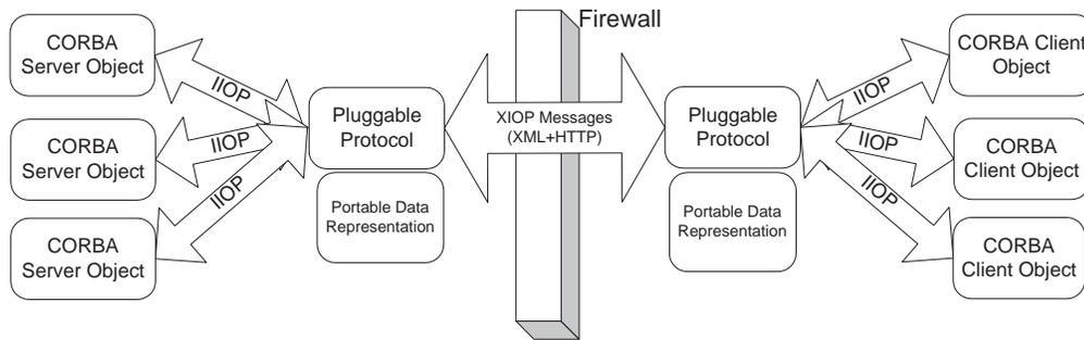
**Figure 2.6:** Diagram showing the mechanism of XIOP
