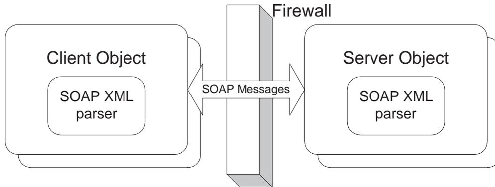
**Figure 2.5:** Diagram showing the mechanism of SOAP
