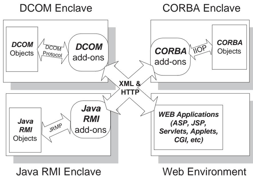
**Figure 5.5:** Allowing heterogeneous systems to communicate
