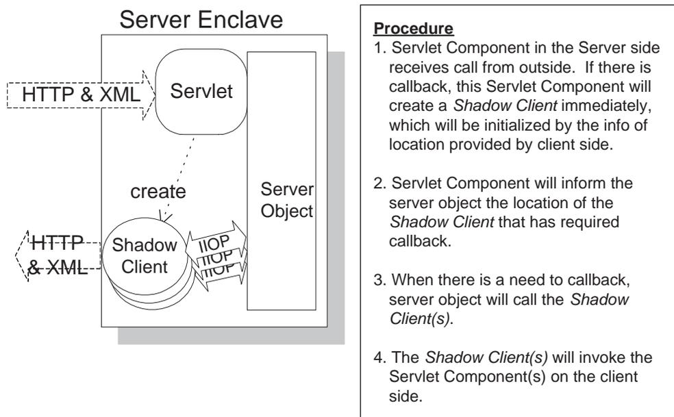
**Figure 3.6:** CORBA callback mechanism in server side
