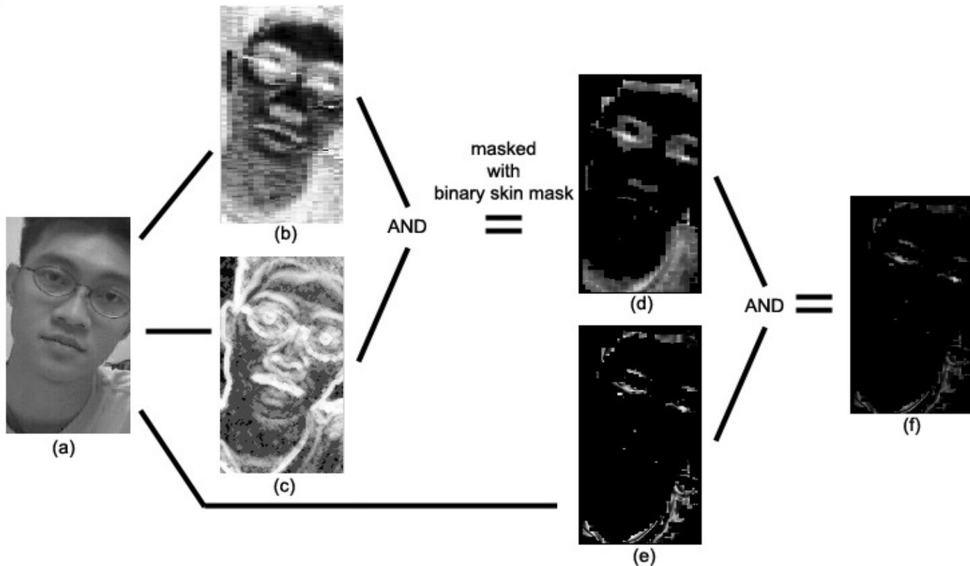
Figure 10: The calculation of EM. (a) The original image, (b) EC after histogram equalization, (c) EL after histogram equalization, (d) the masked intermediate image of ((b) AND (c)), (e) the sepmap SEP, and (f) the resultant eyemap EM.
