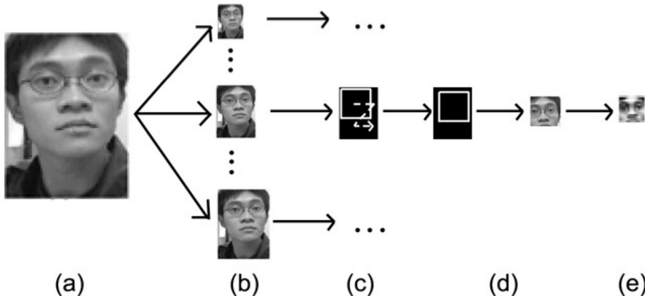
Figure 19: The procedure of face detection: (a) Original face candidate region, (b) resize the region into different scales, (c) the zigzag movement of the 19x19 pixels search window, (d) one of the search window, and (e) histogram equalization on the search window.
