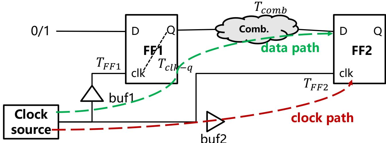
$$T_{FF1} + T_{clk-q} + T_{comb} + T_{setup} - T_{FF2} - T = T_{slack}^{late} \geq 0 \quad \text{Setup Constraint}$$
