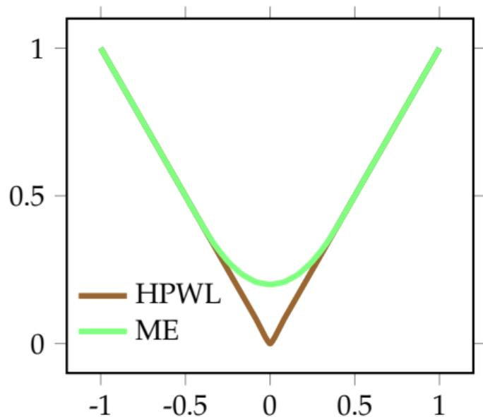
Figure: A simple example of approximating  $\max\{x,0\} - \min\{x,0\} = |x|$  (2-pin net) with ME model, under  $t = 0.2$ .
