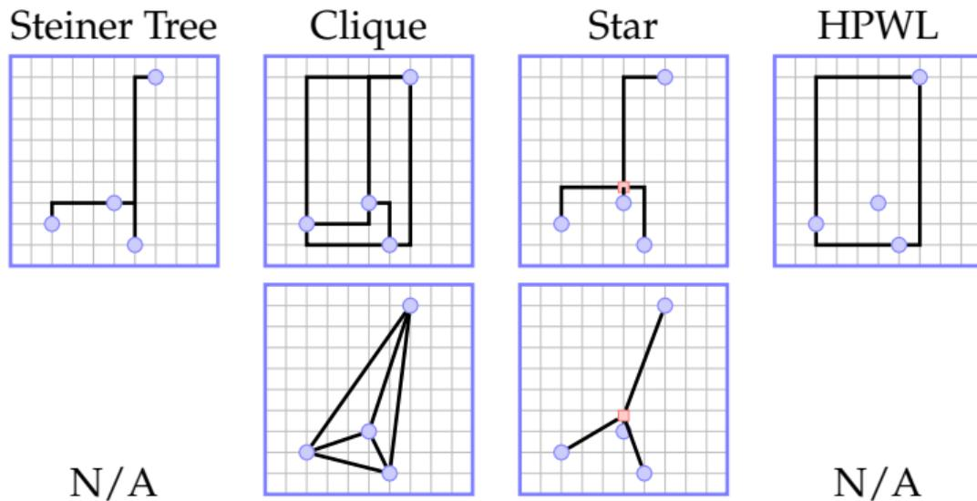
**Table:** Examples of different wirelength models. The first row shows models using  $\ell_1$  distance, while the second shows those using  $\ell_2$  distance.
