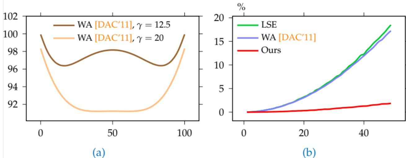
Figure: (a) The non-convexity of WA [DAC'11] on a simple 3-pin net to approximate  $\Delta x = \max\{x_{\min}, x, x_{\max}\} - \min\{x_{\min}, x, x_{\max}\}$ . (b) The average approximation against  $\gamma$  or  $t$  for 4-pin nets, under fixed  $\Delta x = 200$ .
