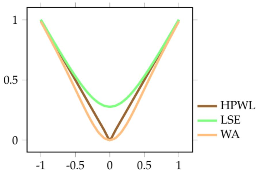
Figure: A simple example of approximating  $\max\{x, 0\} - \min\{x, 0\} = |x|$  (2-pin net) with differentiable models, under  $\gamma = 0.2$ .
