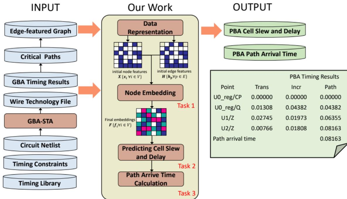
**Cell Features** and **Edge Features** are selected based on circuit knowledge and parameter-sweeping experiments, which can assist EdgeGAT.
