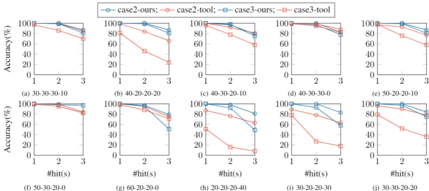
Accuracy of identifying 1, 2, and 3 true root causes in top-3 layout patterns on mixture datasets.
