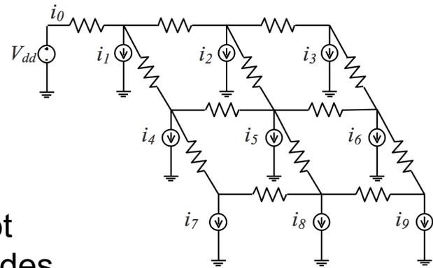
**Problem:** accuracy on the Vdd node does not guarantee accuracy on the current source nodes
