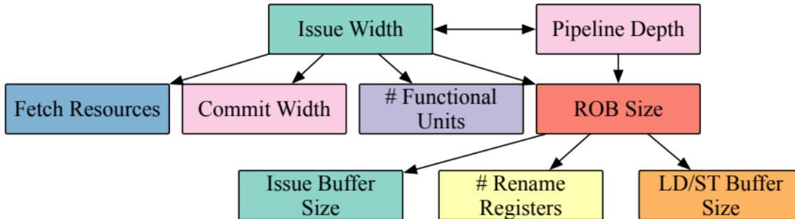
A microarchitecture scaling graph of an example out-of-order microprocessor.
