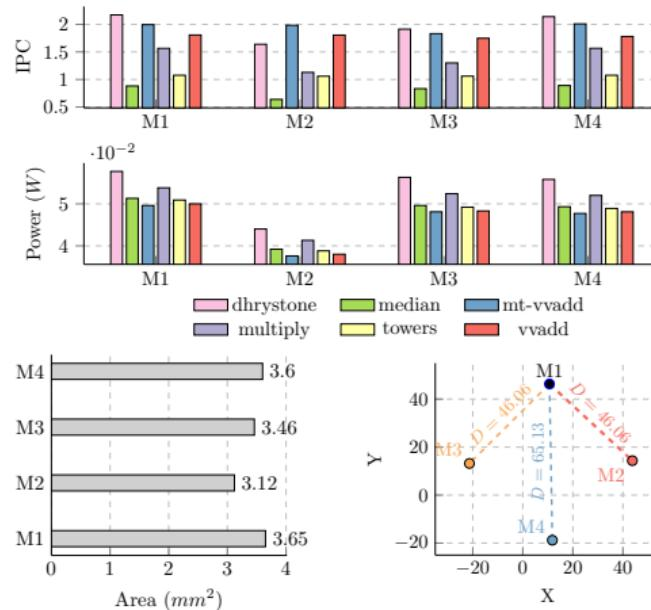
An example of different BOOM microarchitectures to demonstrate the claim.
