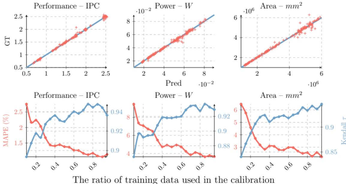
The accuracy of lightweight PPA models, and MAPE and Kendall  $\tau$  curves *w.r.t.* the calibration data size.
