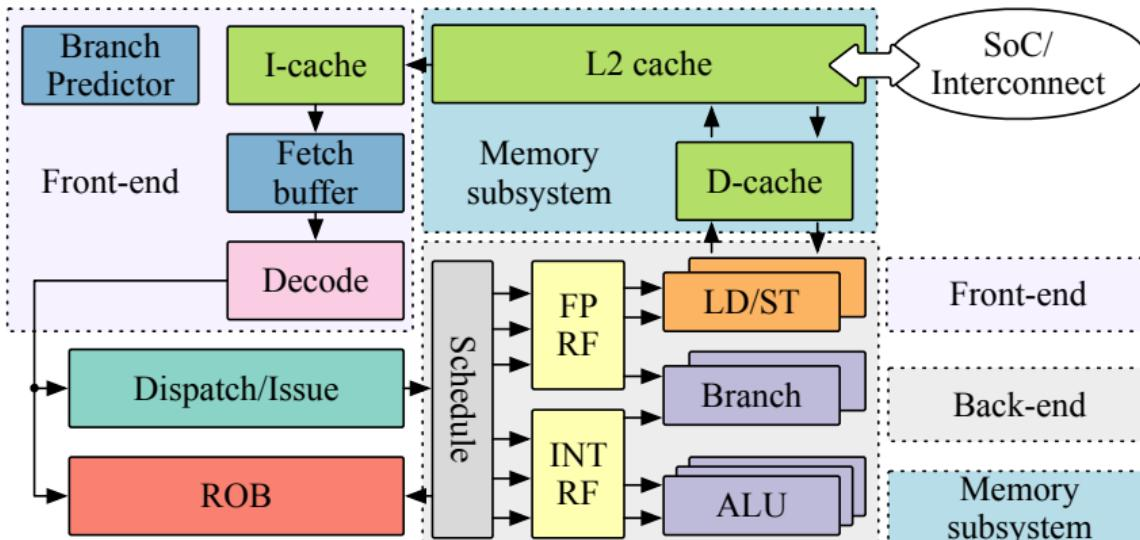
An overview of the example microprocessor microarchitecture, including different *components*.
