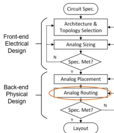
The design flow of analog circuits.
