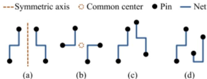
(a) Symmetric constraint. (b) Common-centroid constraint. (c) Topology-matching constraint. (d) Length-matching constraint.
