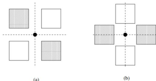
2-D symmetry (b) does not include placement (a) which also satisfies the common centroid constraint.
