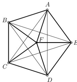
Every thick edge has weight 1, whereas every thin edge has weight 2. Note that the triangle inequality is satisfied. Clearly, an optimal Hamiltonian cycle has length 6, as can be achieved by the cycle  $A \rightarrow B \rightarrow C \rightarrow D \rightarrow E \rightarrow F \rightarrow A$ .
