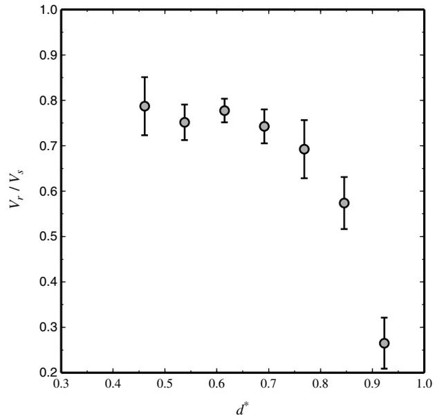
**Figure 4.** Change in the rupture speed  $V_r/V_s$  as a function of down-dip distance  $d^*$ . The rupture speed is computed at the down-dip edge of the seamount, where the rupture has not propagated into the seamount patch yet. Error bars indicate 95% confidence interval calculated for all simulation cases at the same  $d^*$ .
