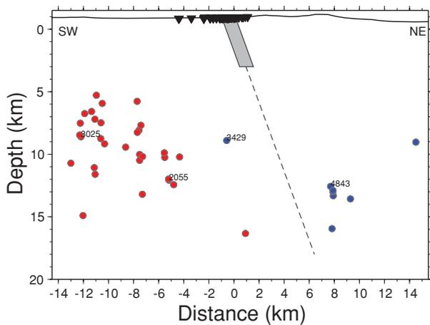
**Figure 8.** A cross-section view of event locations (colour dots) and stations (triangles). Blue and red colours represent positive and negative  $P$ -wave traveltimes differences between the northeastern most and southwestern most stations of the B array, respectively. Grey bar shows the dip and depth of the low-velocity zone obtained in this study.
