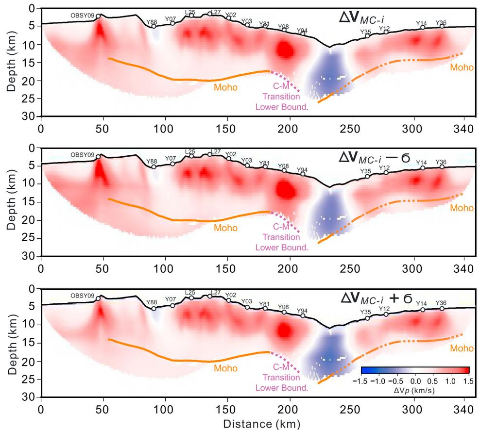
**Figure 5.** (a) Velocity difference  $\Delta V_{MC-i}$  between the Monte Carlo average model (Figure 4a) and the average initial model. (b) Velocity difference  $\Delta V_{MC-i}$  minus the Monte Carlo standard deviation  $\sigma$ . (c) Velocity difference  $\Delta V_{MC-i}$  plus the Monte Carlo standard deviation  $\sigma$ . The low-velocity anomalies beneath the Southwest Mariana Rift (distance of 80–110 km) and near the trench axis (220–250 km) are observed in all three panels.
