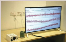
Seismometer and a monitor showing real time ground velocities (ground movement) recorded
