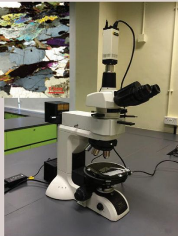
Petrographic Microscope for identifying rocks and minerals in thin sections
