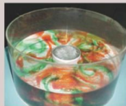
Weather in a Tank for geophysical fluid dynamics (GFD) experiment using a rotating tank
