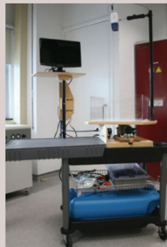
Weather in a Tank for geophysical fluid dynamics (GFD) experiment using a rotating tank
