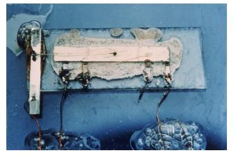
**1958**, by Jack Kilby@Texas Instruments, by hand, several transistors, resistors and capacitors on a single substrate
