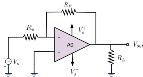
Figure 8: Inverting Amplifier.
