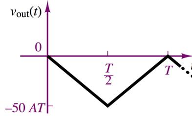
Figure 4: The sketch of output of integrator.
