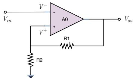
Figure 6: Schmitt Trigger.
