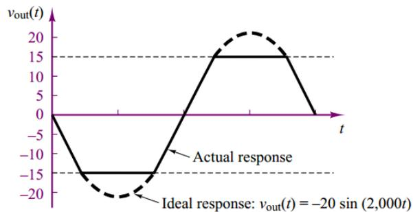
Figure 9: A7. Sketch of output voltage.
