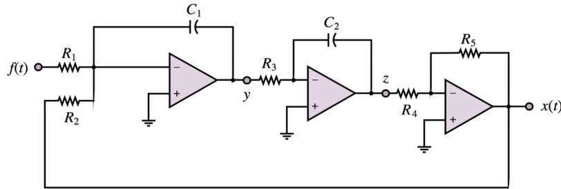
Figure 5: Analog computer simulation of unknown system.
