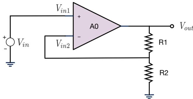
Figure 1: Non-inverting Amplifier.
