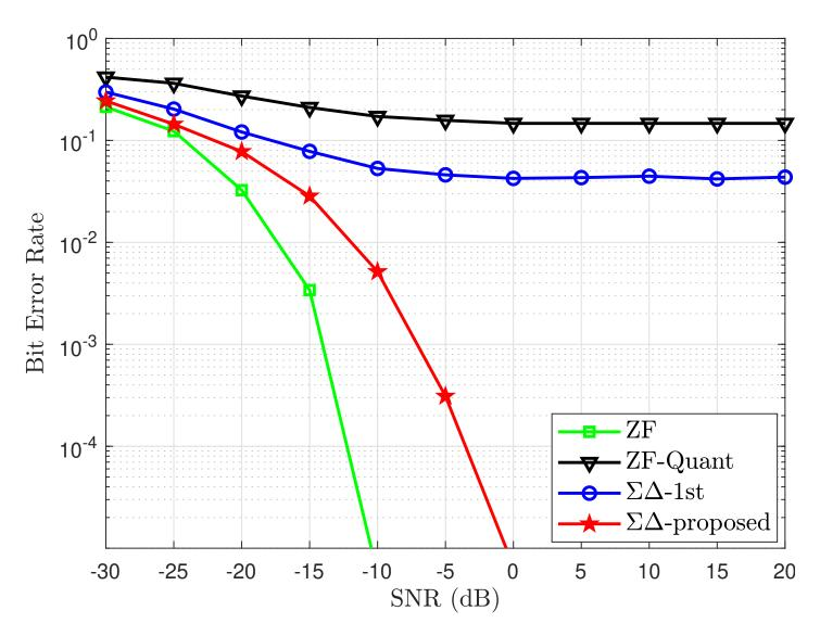
problem size (N,K)=(1024,6), filter order D=24, M=4 quant. levels, antenna spacing  $d=\lambda/2$ , channel gains are randomly generated,  $\theta\in[-70^\circ,70^\circ]$
