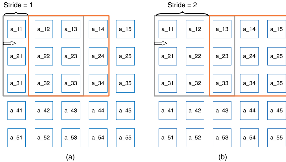
Fig. 3 3 \times 3 convolution example with stride set to (a) 1 and (b) 2, respectively.
