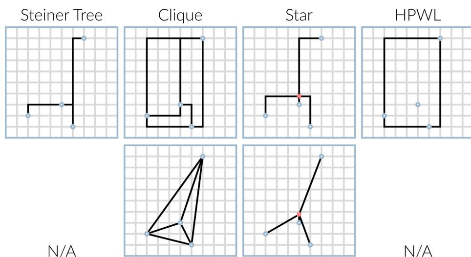
Table 1. Examples of different wirelength models. The first row shows models using  $\ell_1$  distance, while the second shows those using  $\ell_2$  distance.
