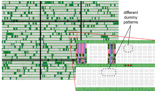
Fig. 18. Possible Locations of inserted dummies on Design C2. Filling windows are marked with black bold lines. Metal wires are colored green and gray rectangles are filled dummies.
