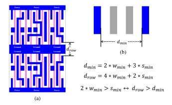
Figure 2: (a) Minimum spacing between M1 wires among different rows. (b) Minimum spacing between M1 wires with the same color.
