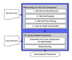
Figure 3: Overall flow of the methodologies for standard cell compliance and detailed placement.
