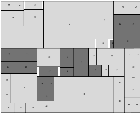
Fig. 7. A result packing of ami49 with four clusters ( C_1 :6,7,8,9; C_2 :10,11,12,13; C_3 :15,16,17,18; C_4 :18,19,20,21)
