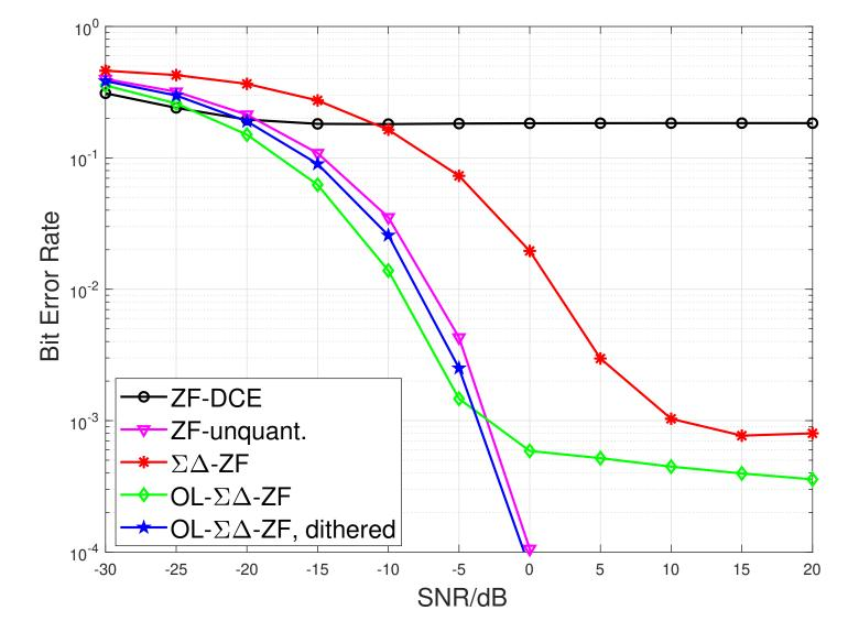
$(N, K) = (512, 8), d = \lambda/8, \theta_{in} = -60^{\circ}, \theta_k \in [20^{\circ}, 40^{\circ}], 16$ -ary QAM; overloaded by  $A = \sqrt{2}$ ; L = 4 discrete phases; dither strength is 0.2A
