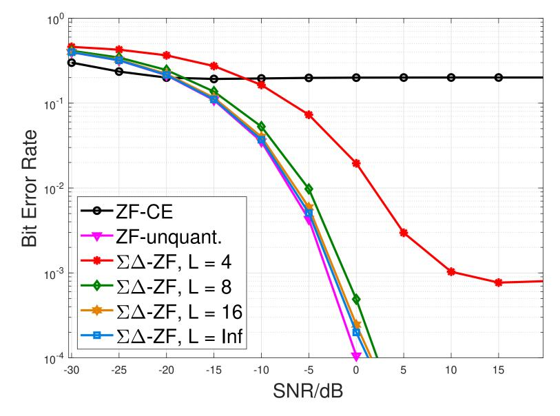
$(N,K) = (512,8), d = \lambda/8, \theta_{in} = -60^{\circ}, \theta_k \in [20^{\circ}, 40^{\circ}], 16$ -QAM; L is the number of discrete phases used
