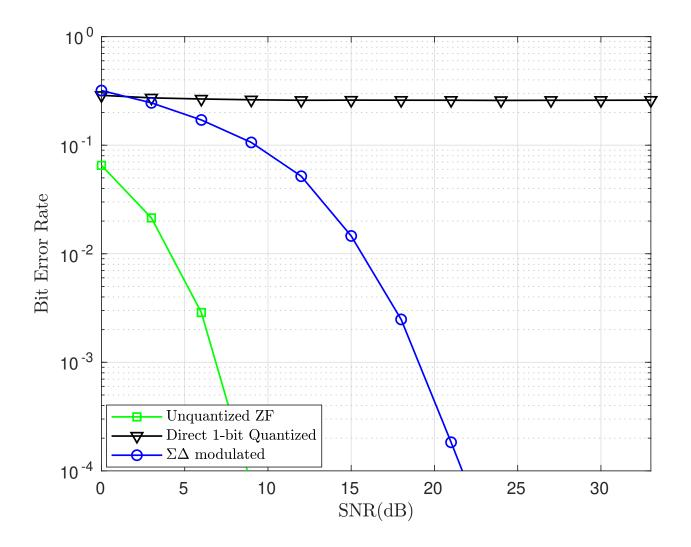
• settings: N = 512 Tx antenna; K = 12 users with  $\theta_k \in [-30^\circ, 30^\circ]$ ; the antenna spacing is set as  $d = \lambda/8$ .
