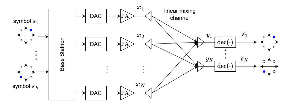
• a simple MU-MISO downlink system  $y_k = \boldsymbol{h}_k^\top \boldsymbol{x} + \text{noise}, \qquad k = 1, \dots, K,$ is the received symbol:  $\boldsymbol{h}_k$  is the channel gain vector
