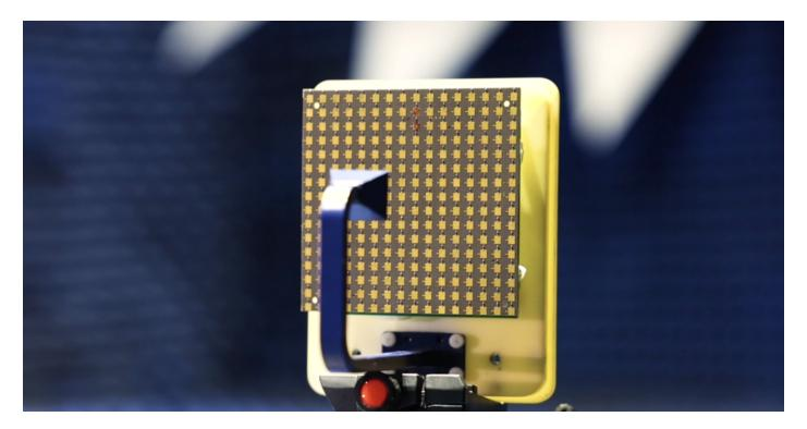
Source: M. Cui, Z. Wu, Y. Chen, S. Xu, F. Yang, and L. Dai, "Demo: Low-power communications based on RIS and AI for 6G," in Proc. IEEE ICC, Dec. 2022.
