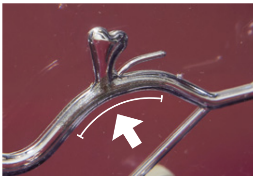
Flow diverter (pipeline) (see arrow)
