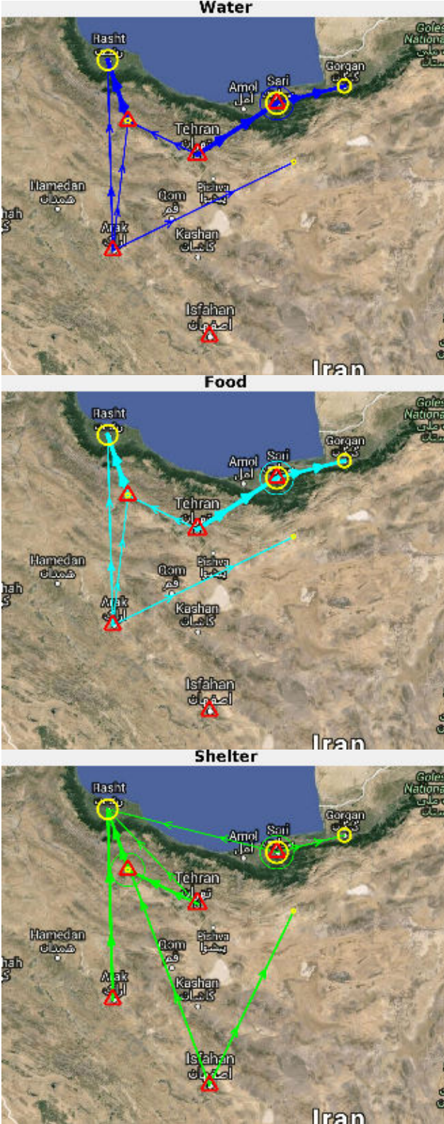
Figure 2 The flows of delivering emergency supplies from storage facilities to affected communities in scenario 1. (Map data: Google)
