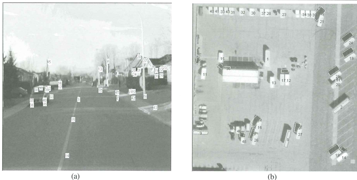
Figure 1. Examples of civil infrastructure objects that can be recognized by Hopfield neural networks: (a) light poles extracted from a mobile mapping image and (b) trucks from an aerial image.
