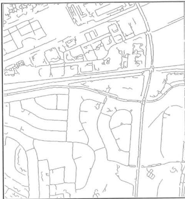
Figure 7. Final road networks obtained using GDPA from figure 5.
