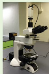
*Petrographic Microscope for identifying rocks and minerals in thin sections
