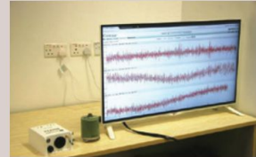
Seismometer and a monitor showing real time ground velocities (ground movement) recorded
