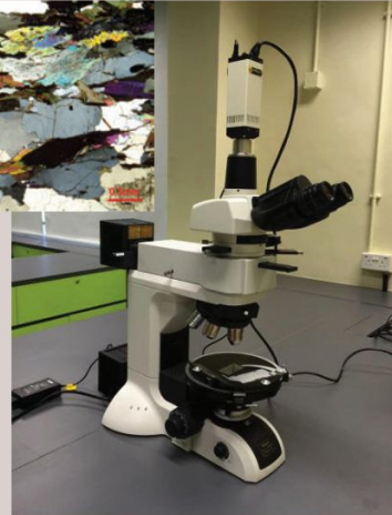
Petrographic Microscope for identifying rocks and minerals in thin sections
