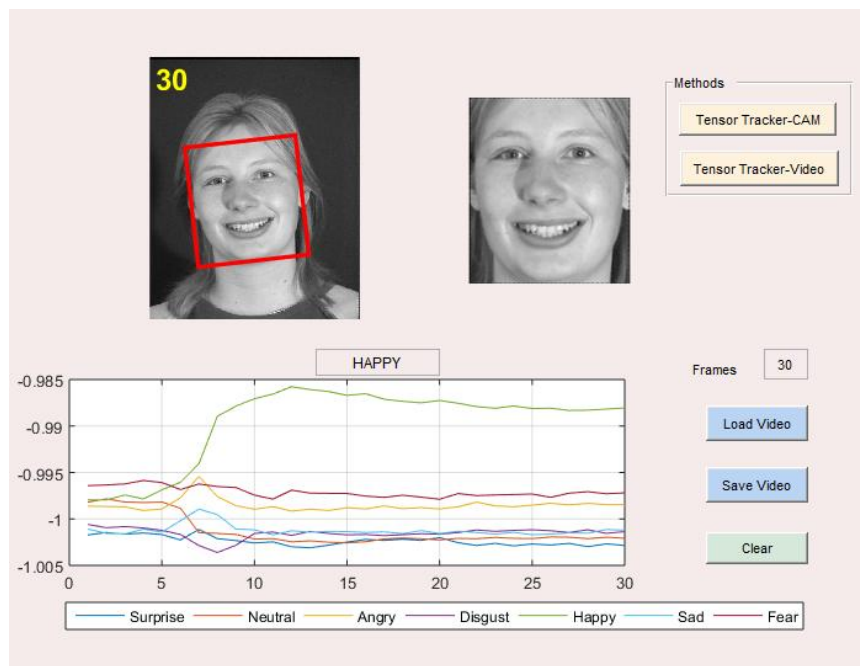
Fig 9: Screen shot of GUI for expression recognition using the proposed tracker for offline videos as well as online ones taken by a camera.
