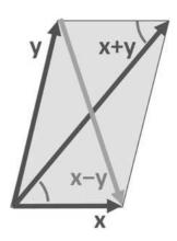
Hence, the geometric meaning is that the sum of the squares of the sides of a parallelogram is the same as the sum the squares of the diagonals
