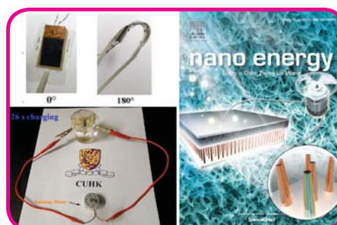
Powering a DC Motor with a Supercapacitor (Zhang et al., Nano Energy, 7, 42-51, 2014)
